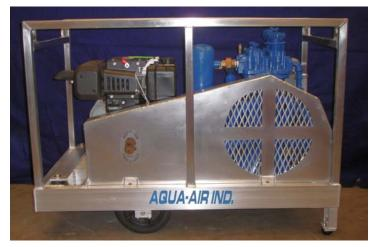
The 325 Air Compressor Package features a Quincy 325, two stage, 2 cylinder, 200psi low pressure compressor with a choice of diesel or gas. Recoil starting is standard. All **Aqua-Air** compressor units feature the Quincy QRB which certifies that the unit has an oil **carry over rating of 2 parts per million.** This American-made product meets the highest standard of workmanship and performance in the industry.
