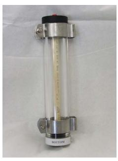
AAI Water Trap is designed to protect the Caisson Gauge that registers external pressure. The water is trapped in an acrylic cylinder so it does not reach the internal parts of the caisson gauge preventing corrosion.
