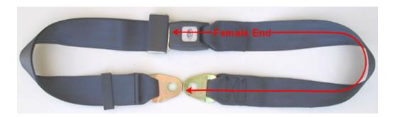
**Non-Retractable Seat Belt** has 2" belt that extends up to 60". These lap belts are manufactured to exceed specifications as set forth by SFI, FIA, USAC, SCCA & FMVSS and are Federal Motor Vehicle Safety Standards (FMVSS) #209 approved. Color provided in Saturation application is "safety orange".
