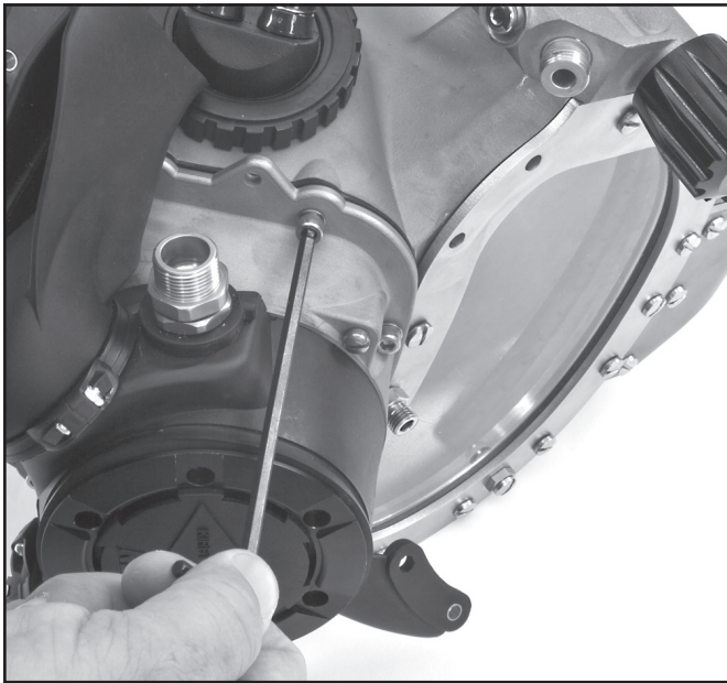
Tighten the nuts in a staggered pattern.
