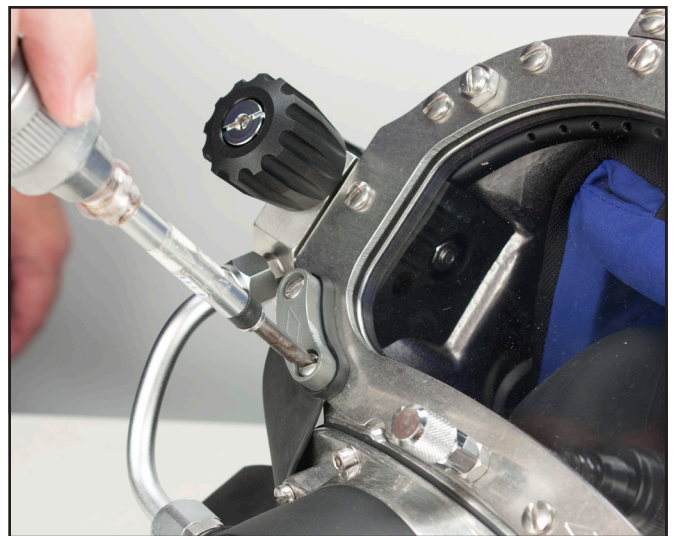
Only use a torque screwdriver to tighten the screws that secure the whiskers to the face port.
