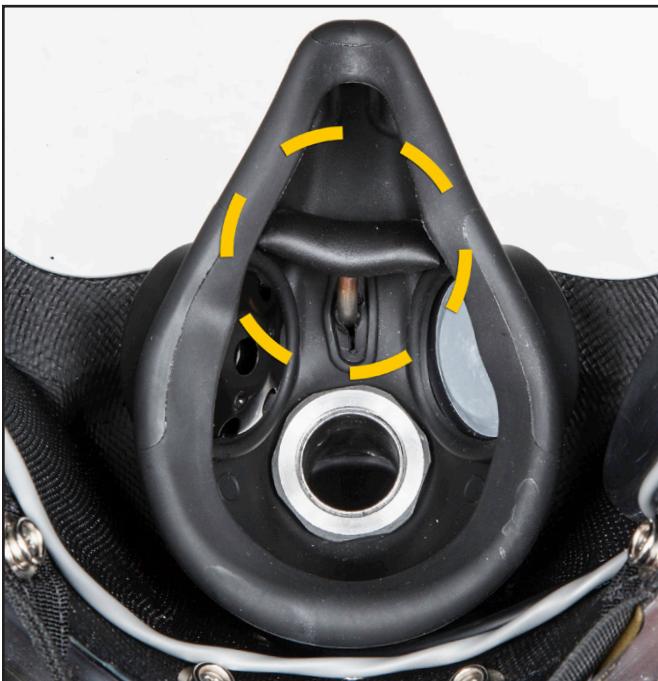
Properly installed nose block device.
