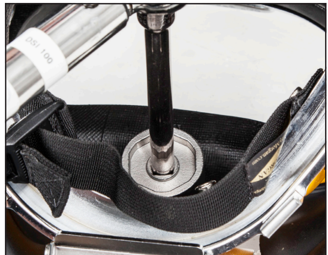
Removal of the regulator mount nut.
