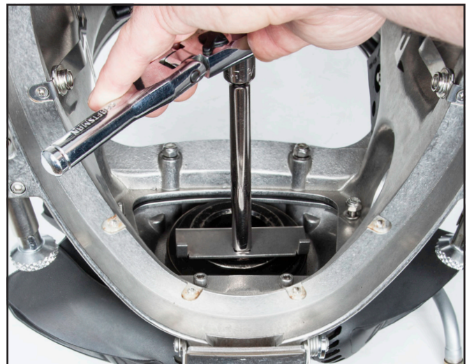
Loosen the regulator for easier removal of the pod screw.
