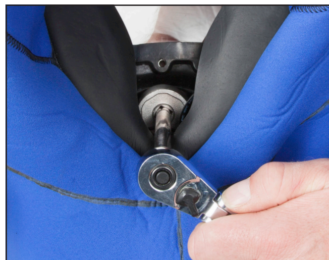
Removal of the regulator mount nut.
