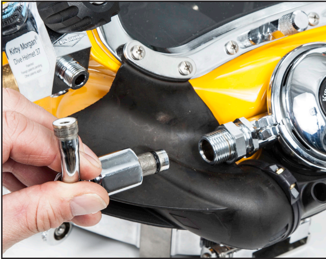
Removing the bent tube.
