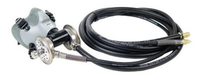
The Avox Pressur-Vak II is designed to administer oxygen or gas mixtures to a diver or patient in a hyperbaric chamber environment. The demand regulator assembly provides breathing gas on demand (inhalation). The regulator is designed to operate with a constant inlet pressure of 65 to 125 psig over chamber pressure.
