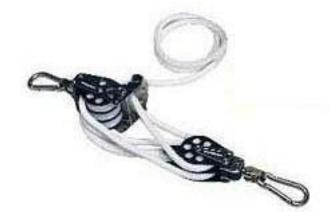
This is the easiest and quickest way to get your crewmember back onboard without the use of a winch. Lifting tackle has a 5:1 purchase, since powerboats generally lack winches, and a triple block with downward facing cam cleat for securing the line.
