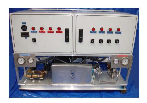
This heater unit is electrically powered and capable of heating seawater and freshwater with a flow of 12 GPM with an adjustable inlet water pressure from 0-15 psi. It has a single boiler heat exchanger.
