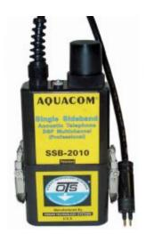
Model: SSB-2010, Aquacom SSB 4-channel, voice menu, diver transceiver.
