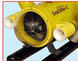
Pan and Tilt Cameras with 100 watts of Lighting
