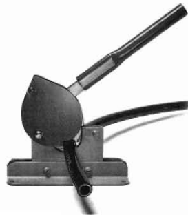
Hose Cutter Part Number: 4523-00000 Use for cutting all sizes of Synflex hose and tubing. The cutter has a spring-actuated guard that holds the hose and protects the operator. Replacement Blade Part Number: 4524-00000
