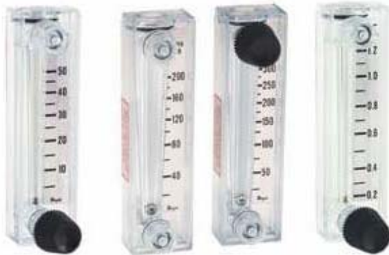
A. Standard Model MMA bottom metering valve. B. Standard Model MMA no valve. C. Standard Model MMA top front mounted metering valve. D. OEM Model MMA. Welded caps on unused valve bosses.
